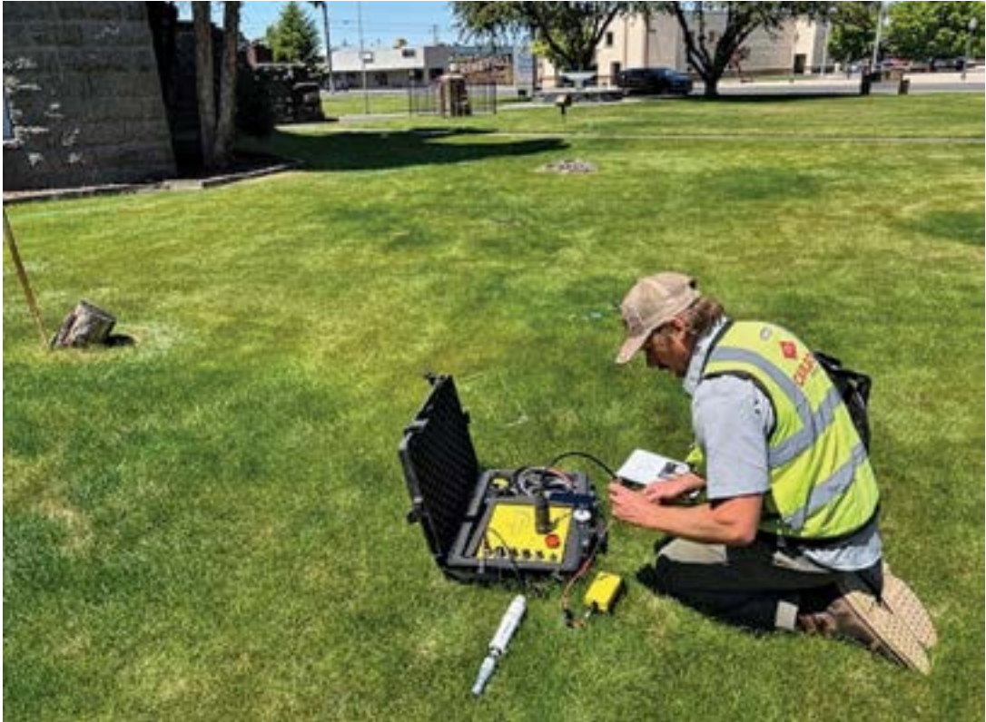
REMI GEOPHYSICAL SURVEY PERFORMED AT LOCAL JOBSITE | PHOTOS COURTESY OF CARLSON TESTING, INC.
